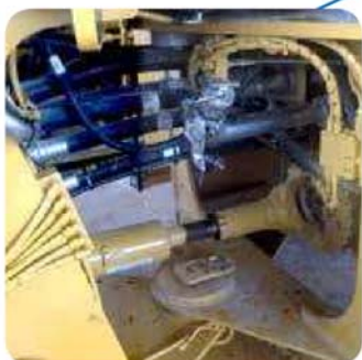
Center pivot area requires proper grease line arrangement to accommodate oscillation
