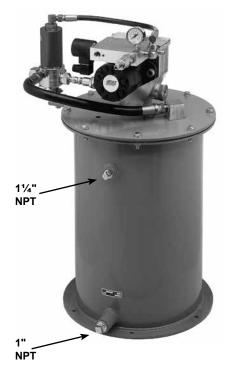
High-performance FlowMaster hydraulic pumps combine rotary-driven pump motors with reciprocating pump tubes and flexible control features that perform in desert heat and arctic cold. Integrated control manifold adjusts the amount of lubricant and operating pressure. The pump's output is adjustable from 7 to 45 cubic inches per minute.
