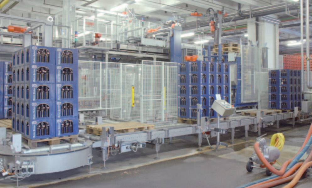
Abb. 3: Palletiser with central lubrication system
