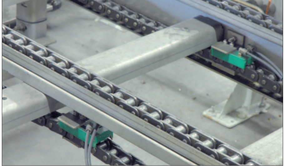
Abb. 4: Lubricated chain conveyor slides over guide rails
