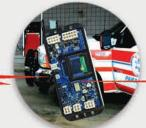
The module transmits the tag ID and vehicle data to the Fuel Management Unit (FMU). The FMU activates the dispenser.
