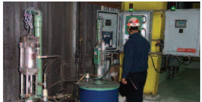
These Lincoln pumps deliver grease directly from a 400 lb. drum to 200 SL-V injectors located approximately 250 feet away in a steel mill.
