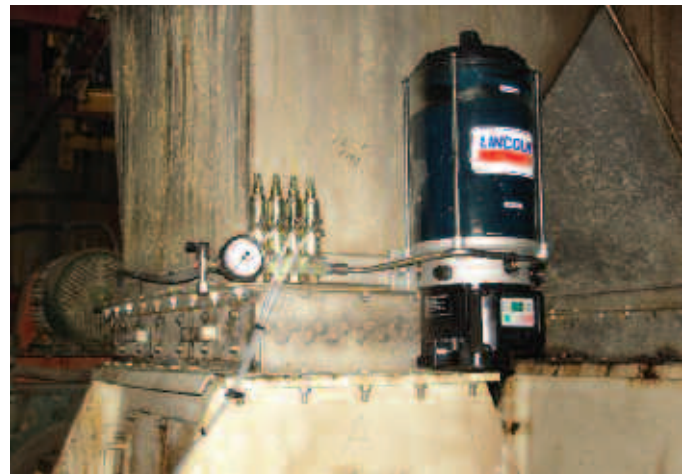
The Centro-Matic Automated Electric Pump and injectors are lubricating bearings in a very abrasive and dusty environment.
