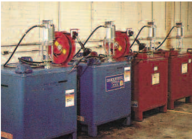
Transferring fluid lubricants and grease from bulk tanks is both cost effective and environmentally sound. These bulk tank systems eliminate drum disposal and the meters will track the volume of lubricant that is dispensed for each product.
