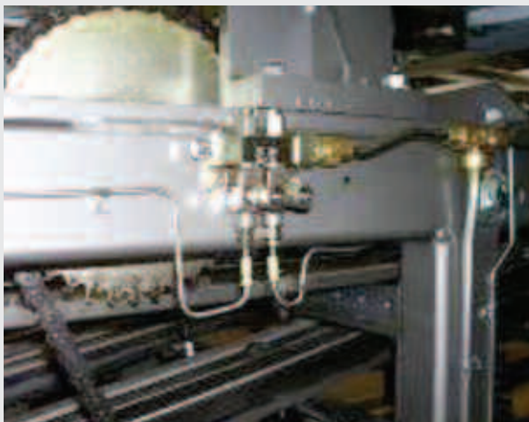
Stainless steel SL-32 grease injectors are used here due to a daily "wash-down" at this food plant.
