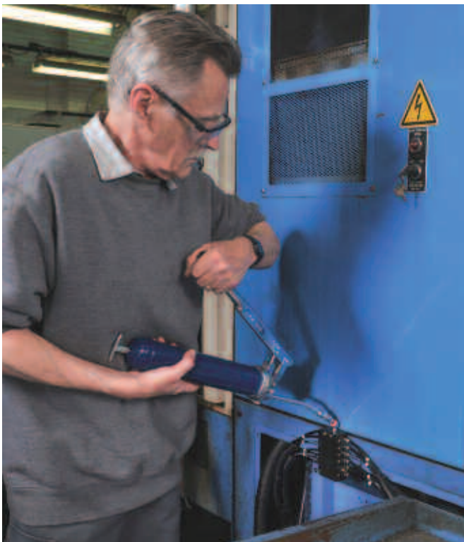
The Single Point Metering Valve enables this technician to lubricate ten bearings without removing any guards or shutting down the production line.
