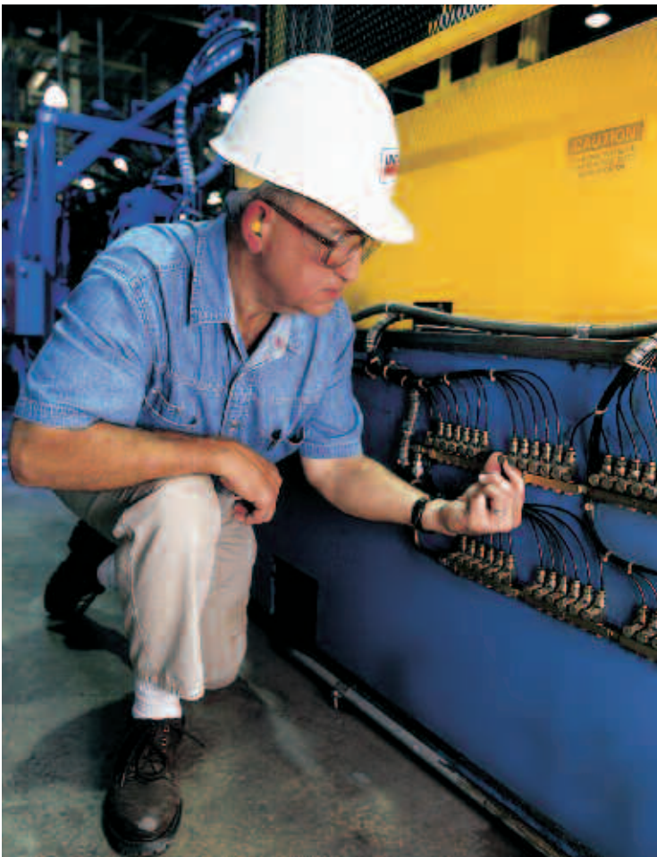
A maintenance technician is adjusting injector output to one bearing on a roll forming machine. More than 100 points are being lubricated from one pump without shutting down the machine.
