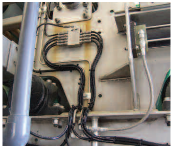
In this corrosive environment, a stainless steel Lincoln Quickclub System is lubricating and purging 32 points on a belt press in a wastewater plant.
