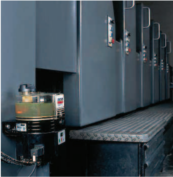
This Lincoln Quickclub QLS Oil System eliminates manual lubrication on bearings and gears for this printing press. Lubricating “on the fly” improves productivity.
