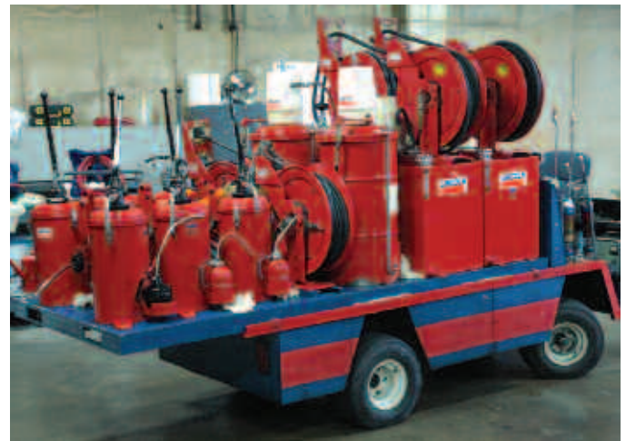
In-plant lube trucks take all the important fluid lubricants to the machinery. This electric cart even includes a waste oil evacuation system.
