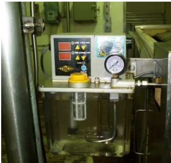
PE-3000 Series Central Lubrication pump mounted on the outside of a pancake process griddle.
