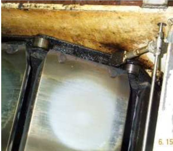
Applicator brush lubricating one of the chains on a pancake process griddle.
